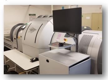
at the airport. The new machine is called a CT-80. Up to this point, all checked bags needed to be individually inspected by hand. More TSA agents and time is required during that process. Now, that is no longer the case. Only bags that alarm through this advanced screener will need
