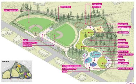
The Loop is the heaviesttouch proposal that the reorientates baseball fields. To do this would require the most movement of dirt to create the best topography for field construction. That would include building a retaining wall. There are three separate plazas athletic, (an community, and teen area).
