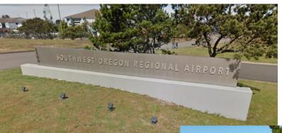
The metal-clad sign has weathered over time from the coastal climate, fading the surface of the sign and corroding the rivets that holds the skin of the sign in place.
